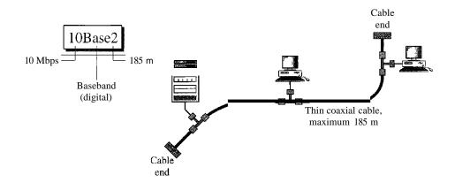
Note that the collision here occurs in the thin coaxial cable. This implementation is more cost effective than 10BaseS because thin coaxial cable is less expensive than thick coaxial and the tee connections are much cheaper than taps. Installation is simpler because the thin coaxial cable is very flexible. However, the length of each segment cannot exceed 185 m (close to 200 m) due to the high level of attenuation in thin coaxial cable.
