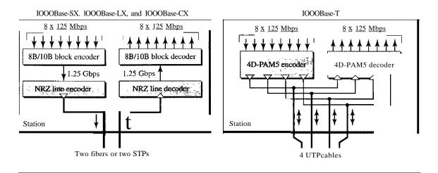
Gigabit Ethernet cannot use the Manchester encoding scheme because it involves a very high bandwidth (2 GBaud). The two-wire implementations use an NRZ scheme, but NRZ does not self-synchronize properly. To synchronize bits, particularly at this high data rate, 8BIIOB block encoding, discussed in Chapter 4, is used.
