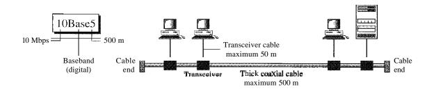
The transceiver is responsible for transmitting, receiving, and detecting collisions. The transceiver is connected to the station via a transceiver cable that provides separate paths for sending and receiving. This means that collision can only happen in the coaxial cable.
