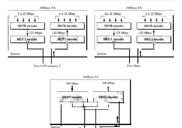
**IOOBase-TX** uses two pairs oftwisted-pair cable (either category 5 UTP or STP). For this implementation, the MLT-3 scheme was selected since it has good bandwidth performance (see Chapter 4). However, since MLT-3 is not a self-synchronous line coding scheme, 4B/5B block coding is used to provide bit synchronization by preventing the occurrence of a long sequence of 0s and Is (see Chapter 4). This creates a data rate of 125 Mbps, which is fed into MLT-3 for encoding.
